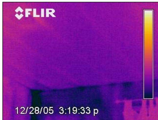
Figure 2.6.2 - Cold air thermal bypass at a porch roof
