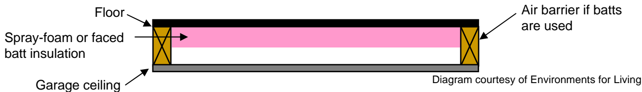
Figure 3.1.3 - Alignment of insulation and air barrier at garage ceiling with spray foam or faced batt insulation
